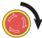
Fig. 1-4: Releasing the emergency stop button by rotating it
