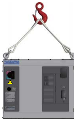
Fig. 3-1: Transport using a crane
