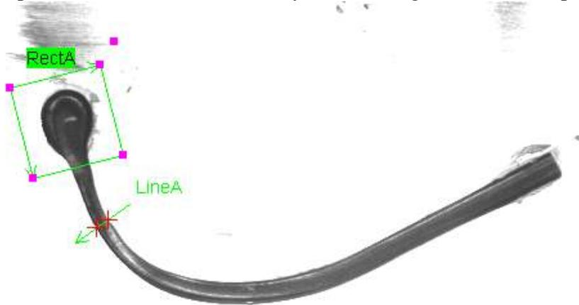
3. Estimate the thickness of the bead where it is thinnest. You can use the mouse or a caliper tool to estimate the bead thickness at the thinnest point. This thinnest point must be 4 or more pixels, as detecting thinner bead widths is unreliable. In the above image, a caliper at LineA was used to estimate the bead thickness. This value will be used for the ***bead thickness*** parameter.
