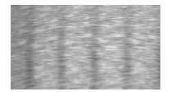
Chatter Edges uses a differentiator filter with an adjustable filter kernel size. For example, a *filter size* of 4 has a kernel of  $\{-1,0,0,1\}$  and one of size 6 has  $\{-1,0,0,0,0,1\}$ . This filter is scanned across the input image, horizontally, vertically or both (*filter direction* parameter) to build up the output image.
