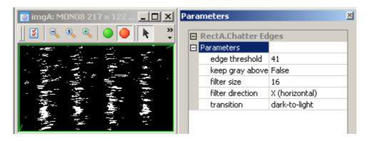
Any output value below *edge threshold* is set to 0. Values at and above *edge threshold* are either output as full white (pixel value = 255) or, if *keep gray above* is True then filter output value above edge threshold are passed unchanged. In the above example, *keep gray* above is False so we get a binary (0 and 255) output image.
